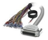
Assembled shielded round cable; connection 1: Single wires (25-position) (The wires are marked and fitted with ferrules. The braided shield is routed to a separate cable end.); connection 2: D-SUB socket strip (1x 25-position); cable length: 2 m
