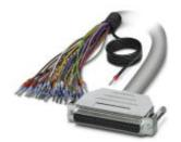
Assembled shielded round cable; connection 1: Single wires (37-position) (The wires are marked and fitted with ferrules. The braided shield is routed to a separate cable end.); connection 2: D-SUB socket strip (1x 37-position); cable length: 2 m
