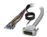
Assembled shielded round cable; connection 1: Single wires (15-position) (The wires are marked and fitted with ferrules. The braided shield is routed to a separate cable end.); connection 2: D-SUB pin strip (1x 15-position); cable length: 0.5 m
