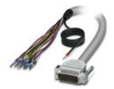
Assembled shielded round cable; connection 1: Single wires (15-position) (The wires are marked and fitted with ferrules. The braided shield is routed to a separate cable end.); connection 2: D-SUB pin strip (1x 15-position); cable length: 3 m
