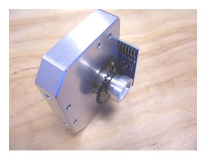
Step 4: Last, connect the two cables. Black wires should be towards the outside and the white wires should be next to each other in the center of the assembly, as shown below.
