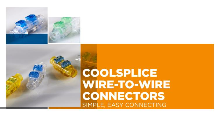
CoolSplice connectors help elimnate the need to pre-strip the insulation from the wire conductors and provide a visually controlled termination. The push connect buttons provides a more ergonomic wire termination than conventional twist-on wire connectors / nuts (marrettes). The slim, symmetrical contoured, snag resistant connectors fit through a 16.00mm [0.630] diameter hole or pvc tube.
