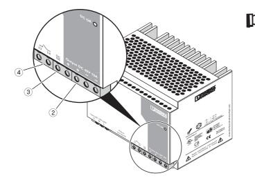
Make sure that all output lines are dimensioned according to the maximum output current or are separately protected. The cables on the secondary side must have sufficiently large cross sections in order to keep the voltage drops on the lines as low as possible.
