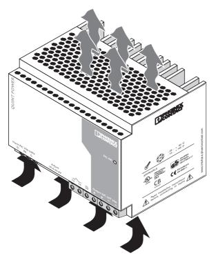
In order to guarantee sufficient convection, we recommend observing the following minimum distance to other modules: 5 cm in a vertical direction and 0 cm in a horizontal direction.
