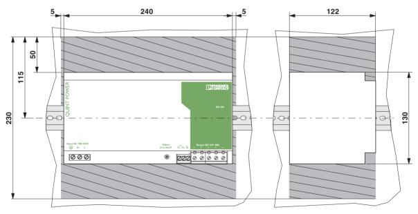
Low-profile installation: Installation depth 125 mm (+ DIN rail)
