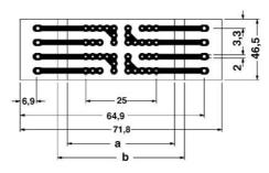
Pitch 5 mm a = Area for mounting components, 38 mm in the hood b = Area for mounting components, 45 mm
