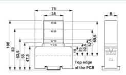
1 = Top edge of the PCB B = Housing width
