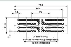
Pitch 5 mm a = Area for mounting components, 38 mm in the hood b = Area for mounting components, 45 mm in the housing
