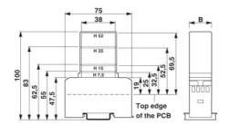
1 = Top edge of the PCB B = Housing width
