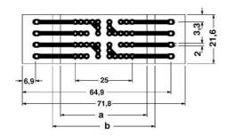
Pitch 5 mm a = Area for mounting components, 38 mm in the hood b = Area for mounting components, 45 mm in the housing
