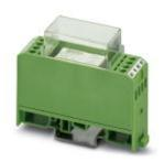
Relay module, with miniature switching relay, with integrated PNP transistor control, for low control currents, contact (AgNi): Medium to large loads, 1 PDT, 12 V DC nominal control voltage
