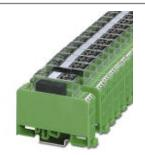
Relay module, with soldered-in miniature switching relay, contact (AgNi): Medium to large loads, double A2 connection, 1 PDT, 120 V AC/DC input voltage
