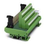
VARIOFACE module, for IEC 603/DIN 41612 connector, type E, 48-pos., a, c, e components mounted, with male connector, cable housing with screw interlock
