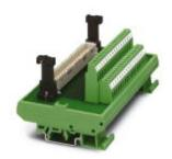
VARIOFACE module, for IEC 603/DIN 41612 connector, type D, 32-pos., a, c components mounted, with socket strip, cable housing with screw interlock
