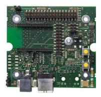
The power to deRFnode and deRFgateway is either supplied by USB, an AC adapter or 3xAA batteries. As programming interface, the standard JTAG connections for ARM and AVR are present together with other standard interfaces like SPI, UART and I2C. Additional sensors for special measurement tasks can be connected using the 34 pin expansion header.
