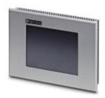
Touch panel with 30.7 cm (12.1") graphics-capable TFT display, 65,535 colors, 800 x 600 pixels, 1 x Ethernet, 2 x USB, and integrated runtime of the Visu+ visualization software.
