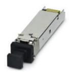
The small form-factor plug-in module is a plug-in fiber optic interface with a data transmission speed of 1000 Mbps, which is used in Gigabit Ethernet. Fiberglass module with a wavelength of 1550 nm (long haul).
