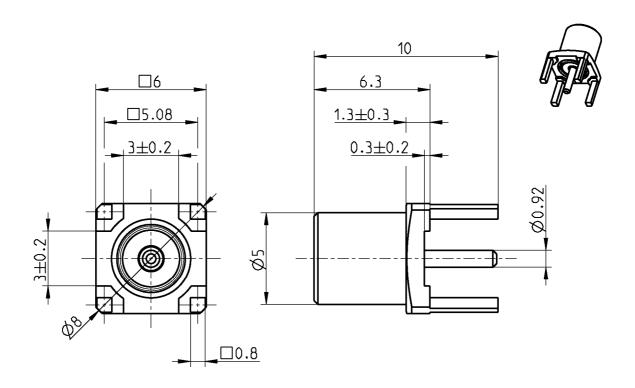
All dimensions are in mm; tolerances acc. ISO 2768 m-H
