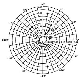
$\begin{array}{l} S_{22e} \\ V_{CE} = 5V \\ I_{C} = 5mA \\ T_{a} = 25^{\circ}C \\ (UNIT:\Omega) \end{array}$
