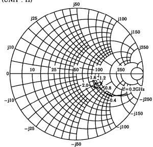
$\begin{array}{l} S_{11e} \\ V_{CE}\!=\!5V \\ I_{C}\!=\!10\text{mA} \\ Ta\!=\!25^{\circ}\!C \\ (UNIT:\Omega) \end{array}$
