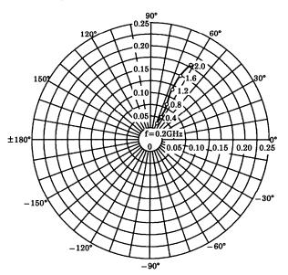
$\begin{array}{l} S_{22e} \\ V_{CE} = 5V \\ I_{C} = 10 mA \\ Ta = 25 ^{\circ}C \\ (UNIT: \Omega) \end{array}$
