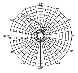
$\begin{array}{l} S_{12e} \\ V_{CE} = 5V \\ I_{C} = 10 \text{mA} \\ Ta = 25^{\circ}C \end{array}$
