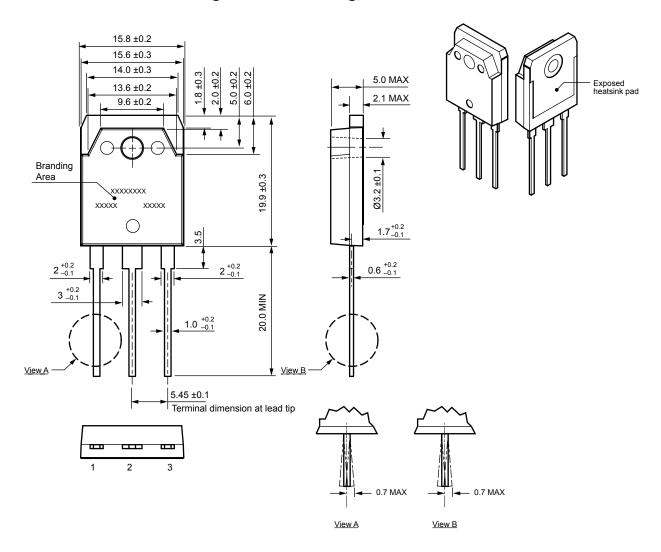
Gate burr: 0.3 mm (max.), mold flash may appear at opposite side Terminal core material: Cu
