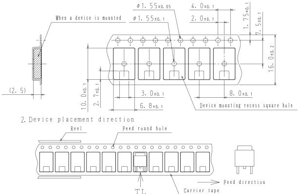
Those with one electrode terminal on the feed hole side ..... TL
