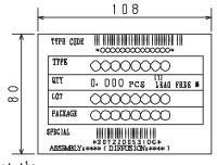
The LEAD FREE \* description shows that the surface treatment of the terminal is lead free.
