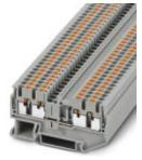
Feed-through terminal block, Connection method: Push-in connection, Number of connections: 4, Cross section: 0.14 mm<sup>2</sup> - 4 mm<sup>2</sup>, AWG: 26 - 12, Width: 5.2 mm, Height: 35.3 mm, Color: orange, Mounting type: NS 35/7,5, NS 35/15
