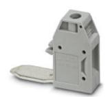
Pick-off terminal block, nom. voltage: 1000 V, nominal current: 57 A, connection method: Screw connection, number of connections: 1, cross section:0.5 mm² - 10 mm², AWG: 20 - 8, width: 10.2 mm, height: 34.7 mm, color: gray, mounting type: on base element
