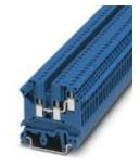
1-level terminal block with double connection on one side, cross section:  $0.2 - 2.5 \text{ mm}^2$ , AWG: 30 - 12, width: 5.2 mm, color: blue
