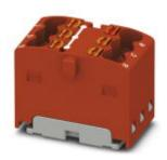
Distribution block, internally jumpered, nom. voltage: 450 V, nominal current: 17.5 A, connection method: Push-in connection, number of connections: 6, cross section:0.14 mm<sup>2</sup> - 1.5 mm<sup>2</sup>, AWG: 26 - 16, width: 12.6 mm, height: 17.6 mm, color: red, mounting type: Direct mounting with flange
