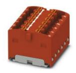
Distribution block, internally jumpered, nom. voltage: 450 V, nominal current: 17.5 A, connection method: Push-in connection, number of connections: 12, cross section:0.14 mm<sup>2</sup> - 1.5 mm<sup>2</sup>, AWG: 26 - 16, width: 25.2 mm, height: 17.6 mm, color: red, mounting type: Direct mounting with flange
