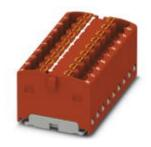
Distribution block, internally jumpered, nom. voltage: 450 V, nominal current: 17.5 A, connection method: Push-in connection, number of connections: 18, cross section:0.14 mm<sup>2</sup> - 1.5 mm<sup>2</sup>, AWG: 26 - 16, width: 37.8 mm, height: 17.6 mm, color: red, mounting type: Direct mounting with flange
