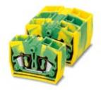
Feed-through terminal block, Connection method: Spring-cage connection, Cross section: 0.14 mm<sup>2</sup> - 2.5 mm<sup>2</sup>, AWG: 26 - 14, Width: 10.4 mm, Height: 9.9 mm, Color: green-yellow, Mounting type: Screw mounting
