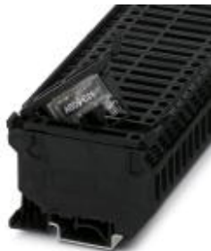
Fuse terminal block for cartridge fuse insert, cross section: 0.2 - 4 mm 2 , AWG: 26 - 10, width: 8.2 mm, color: black
