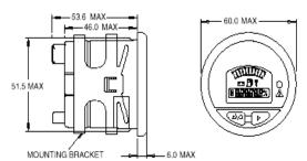
CAUTION: BRACKET IS PLACED OVER GAUGE IN REVERSE FASHION FOR EASE OF SHIPPING. BRACKET HAS BEEN DESIGNED TO REMAIN SECURED TO THE GAUGE UPON PROPER INSTALLATION. ONCE INSTALLED CORRECTLY, ATTEMPTS TO REMOVE BRACKET FROM GAUGE MAY RESULT IN DAMAGE TO THE BRACKET.
