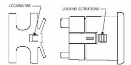
LOCKING TAB MUST ALIGN WITH LOCKING SERRATIONS
