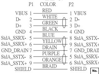
Filler Drain Wire Conductor Jacket FR-PE AL-Foil/Mylar Twist pair AL-Foil/Mylar Braid A-A
