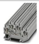
Double-level spring-cage terminal block, for installing components that can be individually selected, nom. voltage: 500 V, nominal current: 22 A, connection method: Spring-cage connection, cross section: 0.08 mm² - 4 mm², AWG: 28 - 12, length: 67.5 mm, width: 5.2 mm, color: gray, mounting: NS 35/7,5, NS 35/15, nom. voltage: 500 V
