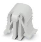
Switching lock, for additional locking of short-circuit switching elements in current transformer measuring circuits, length: 16.3 mm, width: 12.5 mm, height: 13.6 mm, color: white
