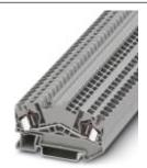
Feed-through terminal block, Connection method: Spring-cage connection, Cross section: 0.08 mm² - 6 mm², AWG: 28 - 10, Width: 6.2 mm, Color: orange, Mounting type: NS 35/7,5, NS 35/15
