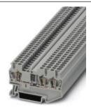
Component terminal block, with integrated diode, Connection method: Spring-cage connection, Cross section: 0.08 mm² - 4 mm², AWG: 28 - 12, Width: 5.2 mm, Color: red, Mounting type: NS 35/7,5, NS 35/15
