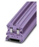
Feed-through terminal block, nom. voltage: 1000 V, nominal current: 24 A, connection method: Screw connection, number of connections: 2, cross section:0.14 mm<sup>2</sup> - 4 mm<sup>2</sup>, AWG: 26 - 12, width: 5.2 mm, color: violet, mounting type: NS 35/7,5, NS 35/15
