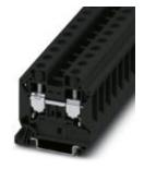
Feed-through terminal block, nom. voltage: 1000 V, nominal current: 76 A, connection method: Screw connection, number of connections: 2, cross section:1.5 mm<sup>2</sup> - 25 mm<sup>2</sup>, AWG: 16 - 4, width: 12.2 mm, height: 54.4 mm, color: black, mounting type: NS 35/7,5, NS 35/15
