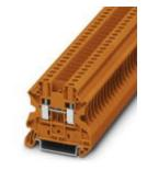
Feed-through terminal block, With breakout partition plate in the bridge shaft, nom. voltage: 1000 V, nominal current: 32 A, connection method: Screw connection, number of connections: 2, number of positions: 1, cross section:0.14 mm<sup>2</sup> - 6 mm<sup>2</sup>, AWG: 26 - 10, width: 6.2 mm, color: orange, mounting type: NS 35/7,5, NS 35/15
