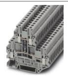
Double-level terminal block, Connection method: Screw connection, Cross section: 0.14 mm² - 4 mm², AWG: 26 - 12, Width: 5.2 mm, Color: black, Mounting type: NS 35/7,5, NS 35/15
