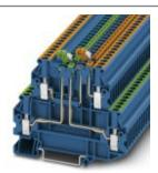
Knife disconnect terminal block, With test socket screws for insertion of test plugs, Connection method: Screw connection, Cross section: 0.14 mm² - 4 mm², AWG: 26 - 12, Nominal current: 16 A, Nominal voltage: 400 V, Length: 80.1 mm, Width: 5.2 mm, Color: blue, Assembly: NS 35/7,5, NS 35/15
