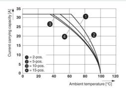
The figure shows the derating curve of the UT 4/1P... terminal block in connection with the UPVB 4 connector
