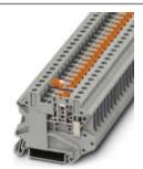
Knife disconnect terminal block, With test socket screws for insertion of test plugs, nom. voltage: 500 V, nominal current: 20 A, connection method: Screw connection, cross section: 0.14 mm² - 6 mm², AWG: 26 - 10, length: 57.8 mm, width: 6.2 mm, color: gray, mounting: NS 35/7,5, NS 35/15, nom. voltage: 500 V/
