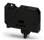
Fuse plug, fuse type: Sand filled, connection method: Plug connection, nominal current: 10 A, nom. voltage: 500 V, width: 8.2 mm, fuse type: G / 5 x 20, color: black
