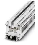
1-level terminal block with double connection on one side, cross section:  $0.2 - 4 \text{ mm}^2$ , AWG: 24 - 12, width: 6.2 mm, color: White
