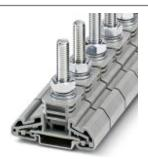
High Current Connectors, nom. voltage: 1000 V, nominal current: 269 A, connection method: Bolt connection, number of connections: 1, width: 32 mm, height: 73.5 mm, color: gray, mounting type: NS 35/7,5, NS 35/15
