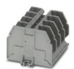
Feed-through terminal block with bolt connection method, cross section: 0.1 - 10 mm<sup>2</sup>, AWG: 26 - 8, width 13 mm, color: gray
