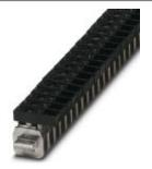
Connection terminal block, Connection method Screw connection, Load current : 41 A, Cross section: 0.5 mm² - 6 mm², Width: 7 mm, Color: green
