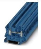
Feed-through terminal block, nom. voltage: 800 V, nominal current: 24 A, connection method: Screw connection, number of connections: 2, cross section:0.14 mm<sup>2</sup> - 4 mm<sup>2</sup>, AWG: 26 - 12, width: 5.2 mm, color: blue, mounting type: NS 35/7,5, NS 35/15
